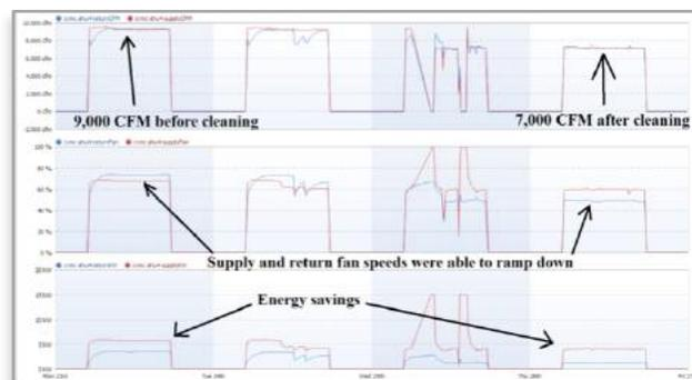
Once identified, cleaning the pitot tube sensor allowed the airflow station to read accurate airflow and the fan VFDs were able to ramp down. Result: energy savings of \$1,300/year for about 15 minutes of cleaning for an issue that would likely have never been detected manually.
