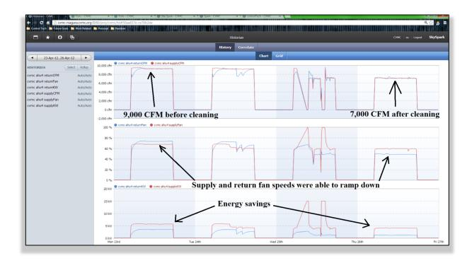
After cleaning the pitot tubes SkySpark® was used to calculate the energy saved. In the first week alone there was a reduction of 250 kWh. Assuming a 52 week hospital year that is 13,000 kWh saved or at \$0.10 a kWh \$1,300 in savings from about 15 minutes of cleaning. SkySpark® can quickly calculate and report savings from simple PM measures that would normally require metering or a measurement and verification process
