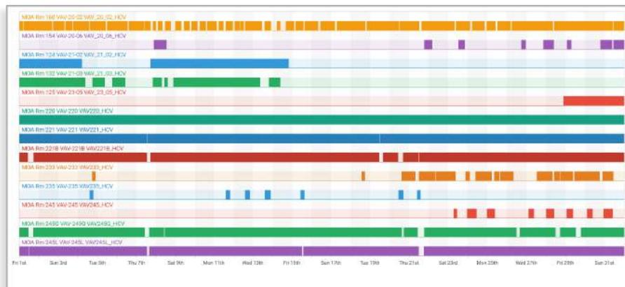
Based on this analysis, 31 reheat valves were replaced in six batches from March 2019 to October 2020. The HRC is now running much more effectively as can be seen in the chart below.
