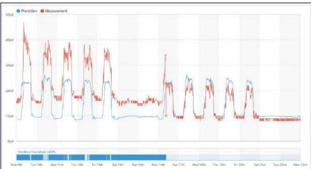
In the view above, we can see the correction of the energy consumption issue after resolution of the issue identified by the Spark Rule
