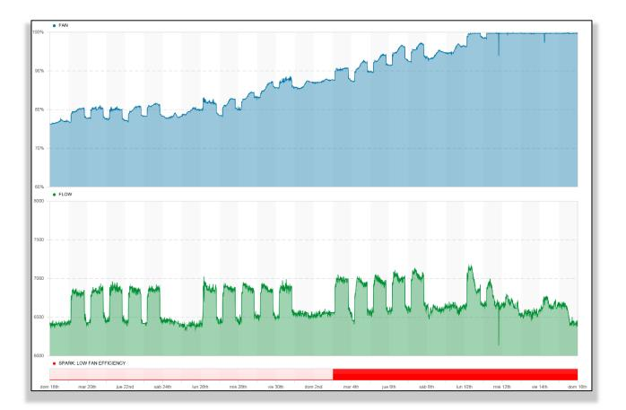
In these SkySpark screens, the Spark (red) shows periods of time where low fan efficiency was detected
