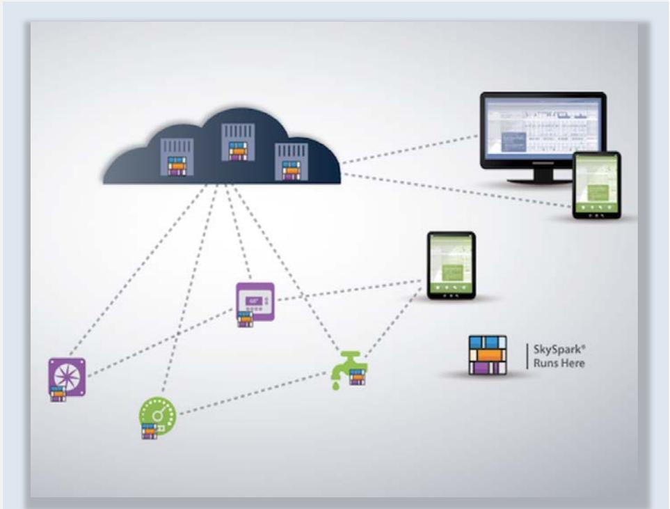
In this architecture SkySpark is installed on small “edge computing” platforms (IoT gateways and OEM controller products) that directly control, manage and analyze data from equipment systems, smart devices or sensors. Every node can provide local user access to all of the capabilities and Apps of SkySpark.
