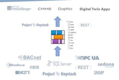
One of the new areas of technology gaining traction in the built environment is "digital twins". The term conveys the concept of a digital representation of a facility implemented via a software application. The representations can extend from the physical structure of the building to the actual data produced by the equipment systems that maintain the occupant environment, and the energy and resource flows associated with those systems.
