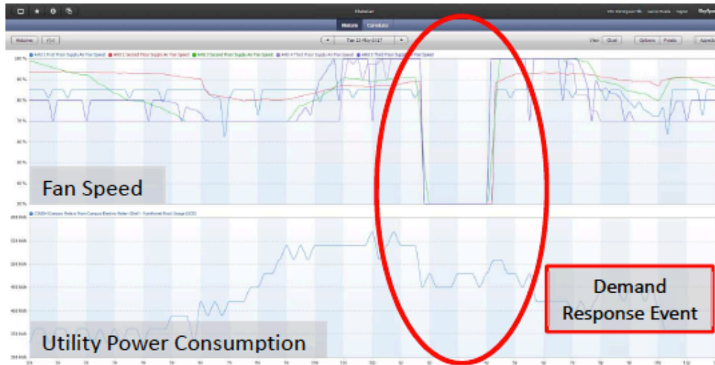
FDD helps CSUDH ensure systems operate as intended during and after demand response events
