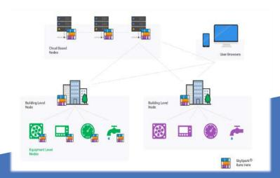
**Distributed Architecture** – By this we mean that SkySpark can be deployed on multiple nodes (computing devices) distributing the work of data collection, analytics processing and presentation of results to users.
