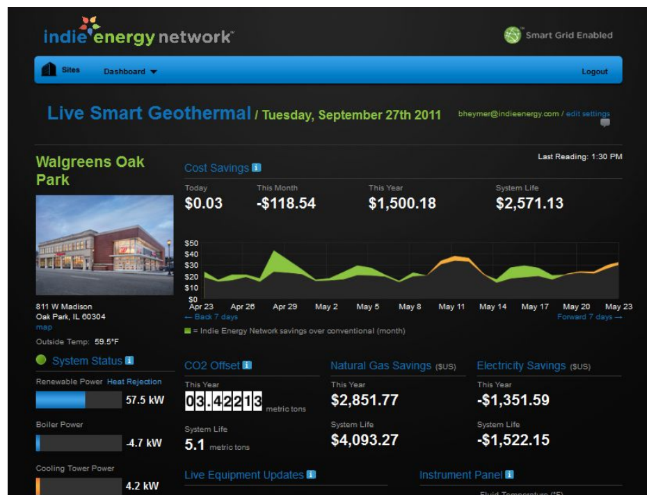
Web-based M&V interface displaying various energy source contributions, cost savings, and environmental benefits resulting from operating the HyGCHP system instead of the conventional HVAC design
