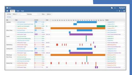
FDD is one subset of the overall capabilities provided by data analytics. This image shows fault patterns as timelines
