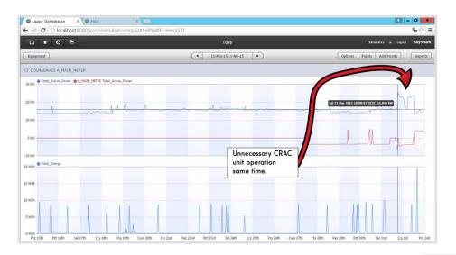
← Here SkySpark shows that both Crac units started at the same time for no reason. The control system sequence was reviewed and modified to correct both issues.
