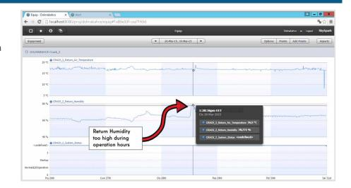
identify and data center facilities staff are empowered to take faster action to avoid potential over-heating that would lead to server failures and downtime.
